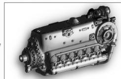
·Type: 12 cylinders in inverted-V layout, water-cooled,
