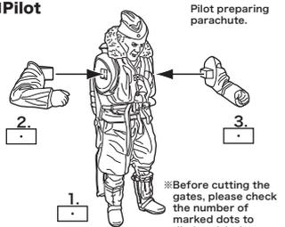
※ Before cutting the gates, please check the number of marked dots to distinguish the parts.
