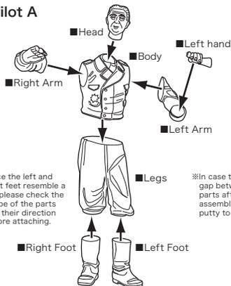
Since the left and right feet resemble a lot, please check the shape of the parts and their direction before attaching.
