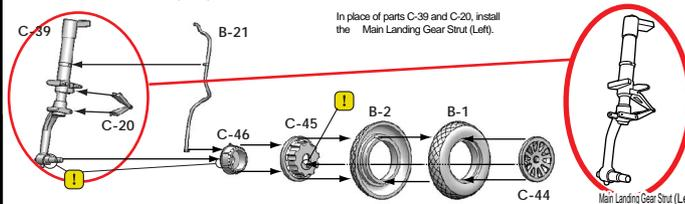
In place of parts C-39 and C-20, install the Main Landing Gear Strut (Left).
