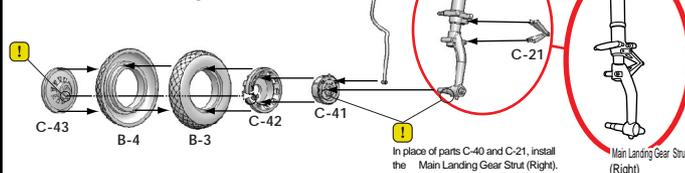
In place of parts C-40 and C-21, install the Main Landing Gear Strut (Right).
