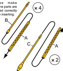
If a part gets stuck during the process of insertion, most likely there are burrs inside the barrel shaft. Please do not force them through, as damage may occur to the parts. Instead, use a 1mm drill bit to smooth out any burrs on the inside of the shaft before resuming building.
