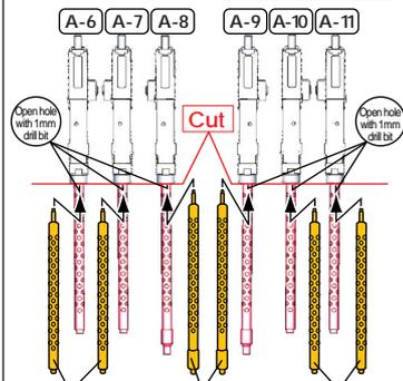
Cut the barrels off of the machine gun parts (A-6, 7, 8, 9, 10, 11) at the red line in the diagram, then use a 1mm drill bit to open holes into which the metal barrels can be inserted, as indicated in the diagram.
