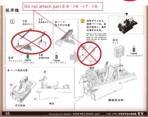
SWS No.01 Shinden Assembly Manual Pages 16-17 3-3. Main Structure and Machine Guns Do not attach any of the parts (machine guns) listed
