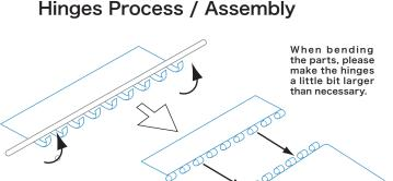
Process the pectinate area that needs to be put together, and assemble. Use a 0.5mm diameter brass pipe (sold separately) to recreate the circular shape of the hinges. Assemble after processing the parts on both sides.
