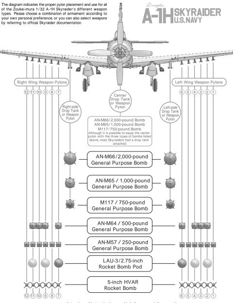
It is not possible to attach every kind of weapon at the same time. Only 4 LAU-3/2.5-inch rocket bomb pods are included in this set. They can be attached at pylons and , and , or and
