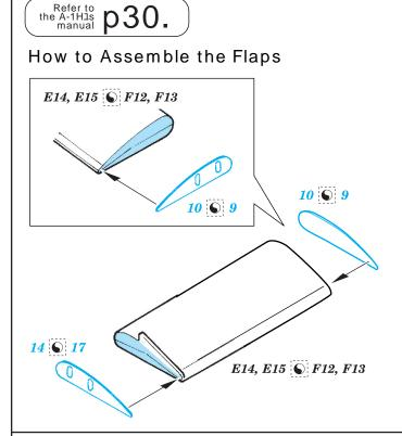
Attach the photo-etched parts to the inner sides only of the right and left ailerons.
